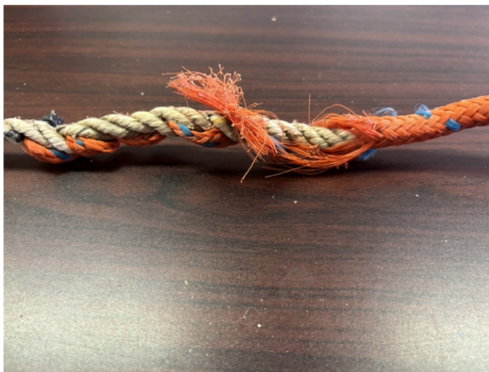
Figure 6.4: Novabraid configuration. The tan rope is inserted into the orange Novabraid.
