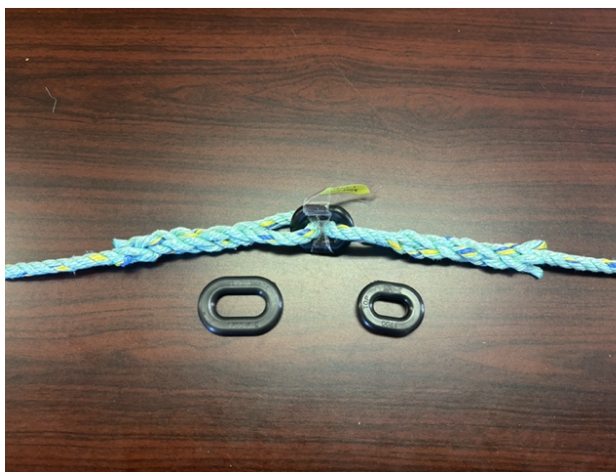
Figure 6.2: Plastic links between two lines. Plante link on left, Brooks link on right.
