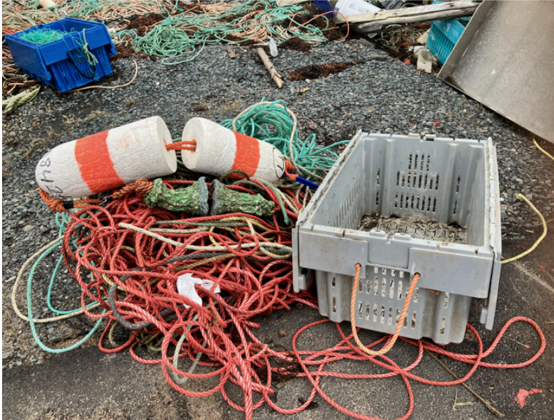
Figure 3: In white and red, some new large buoys. In green below them, the same buoy type after being snarled on the bottom, and crushed by water pressure.
